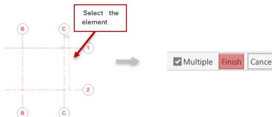
Example of Magnetizing to Grid
