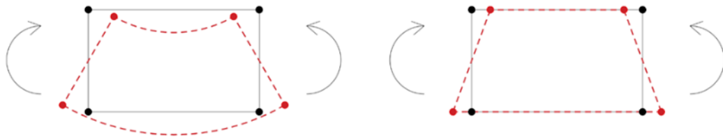
Comparison between real deformation (left) and Q4 element deformation (right)
