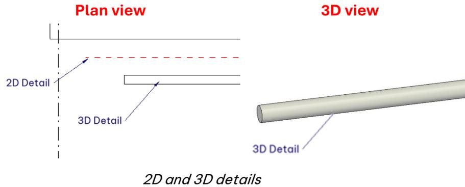
These details items will be created under the detail line for 2D and as a component for 3D details. Therefore, 2D details are visible only in the created view, while 3D details are visible across all intersecting views.
